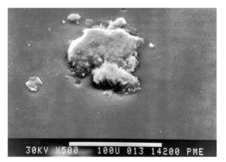
Figure 2. SEM image at 500X of bottom surface glass deposit.
